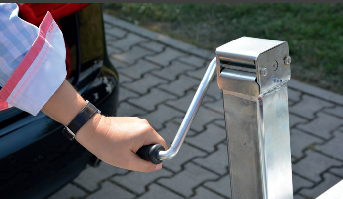
The tipping bridge can be easily brought into the desired position using the hand crank.
