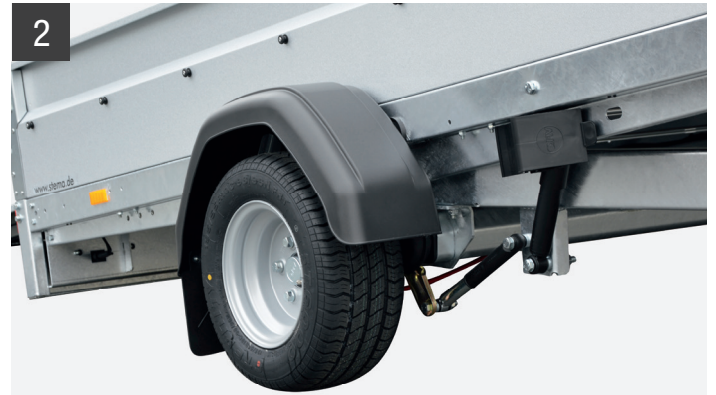
During vehicle loading/unloading, the centre of gravity shifts. This causes the tipping bridge to rise or lower
