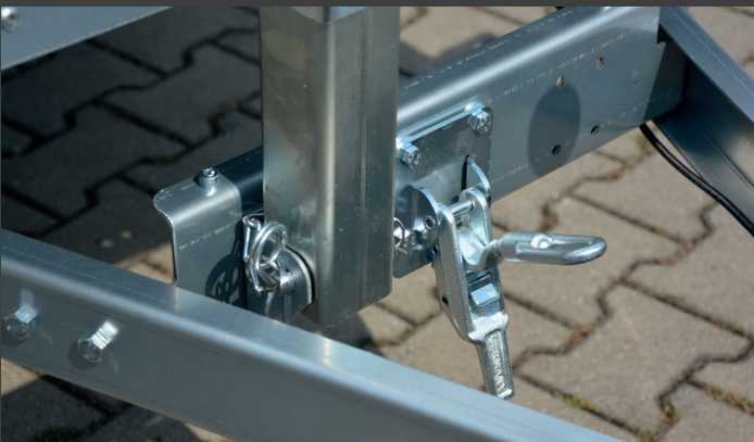
Tipping bridge secured with a locking clamp.
