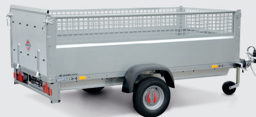
REX with half-open mesh side panel – 66 cm high
