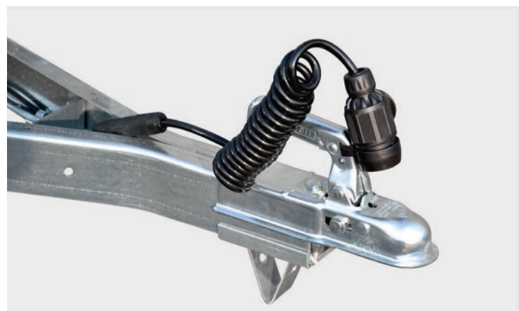
spiral cable with 13-pin connector for flexible connection to the towing vehicle (EC-equipment)
