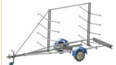
N7-17 kj: Construction for transporting kayaks
