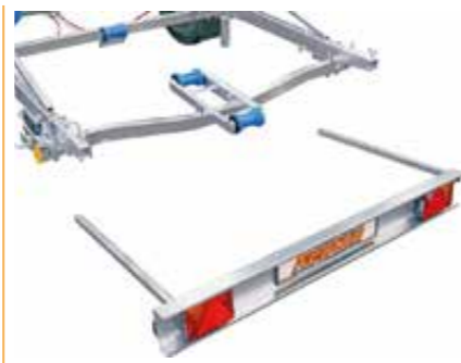
N13-20 navy: Rear Lighting Beam
